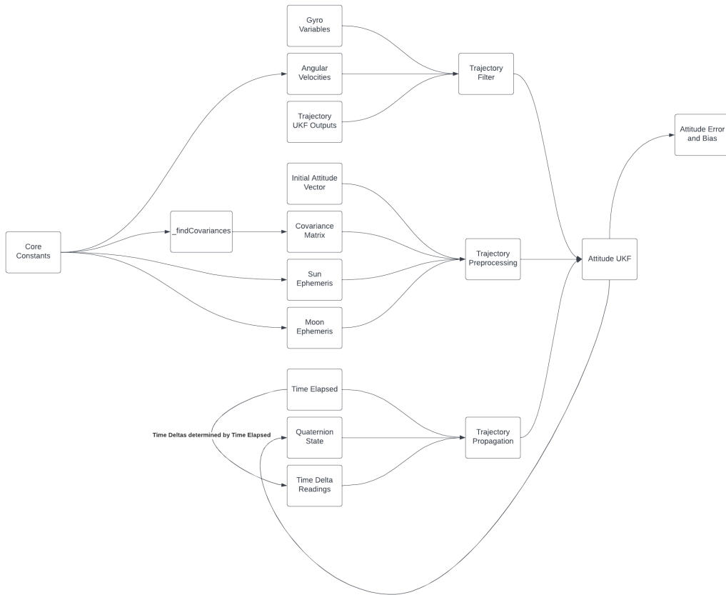
Figure 4: Breakdown of attitude UKF inputs, outputs, and individual component relationships.
